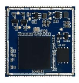
AI face recognition module 3D binocular camera live detection and discrimination serial communication
